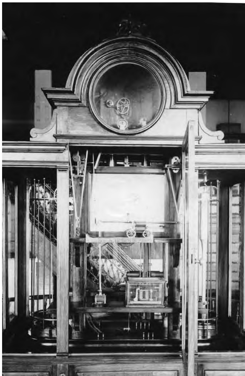
Padre Faura. Third floor of central tower. The Secchi meteorograph obtained by Fr. Faura from Fr. Secchi.
