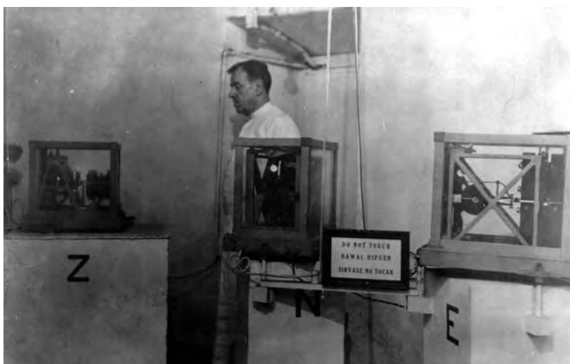
1940. Fr. W. Repetti with the three Gautzin-Wilip seismometers.
